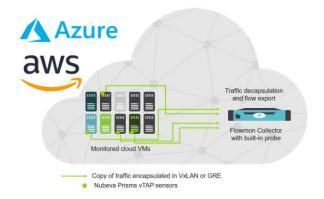
In case where L7 visibility is not required, Nubeva can provide IPFIX or NetFlow directly to Flowmon Collector. Customers optimizing charged data transfers between DCs in different regions can reduce traffic at 500:1 aggregation rate when sending IPFIX/NetFlow instead of mirrored traffic.
